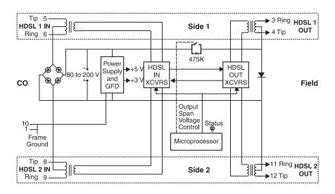
Figure 4. Doubler Block Diagram
